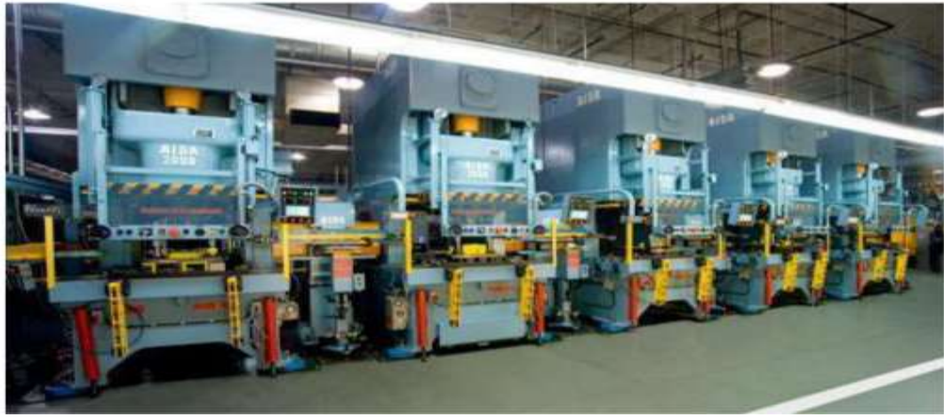
Figure 26 Example of 20 stations Transfer line
